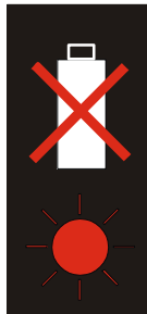
Red flashing (h) Faulty battery
