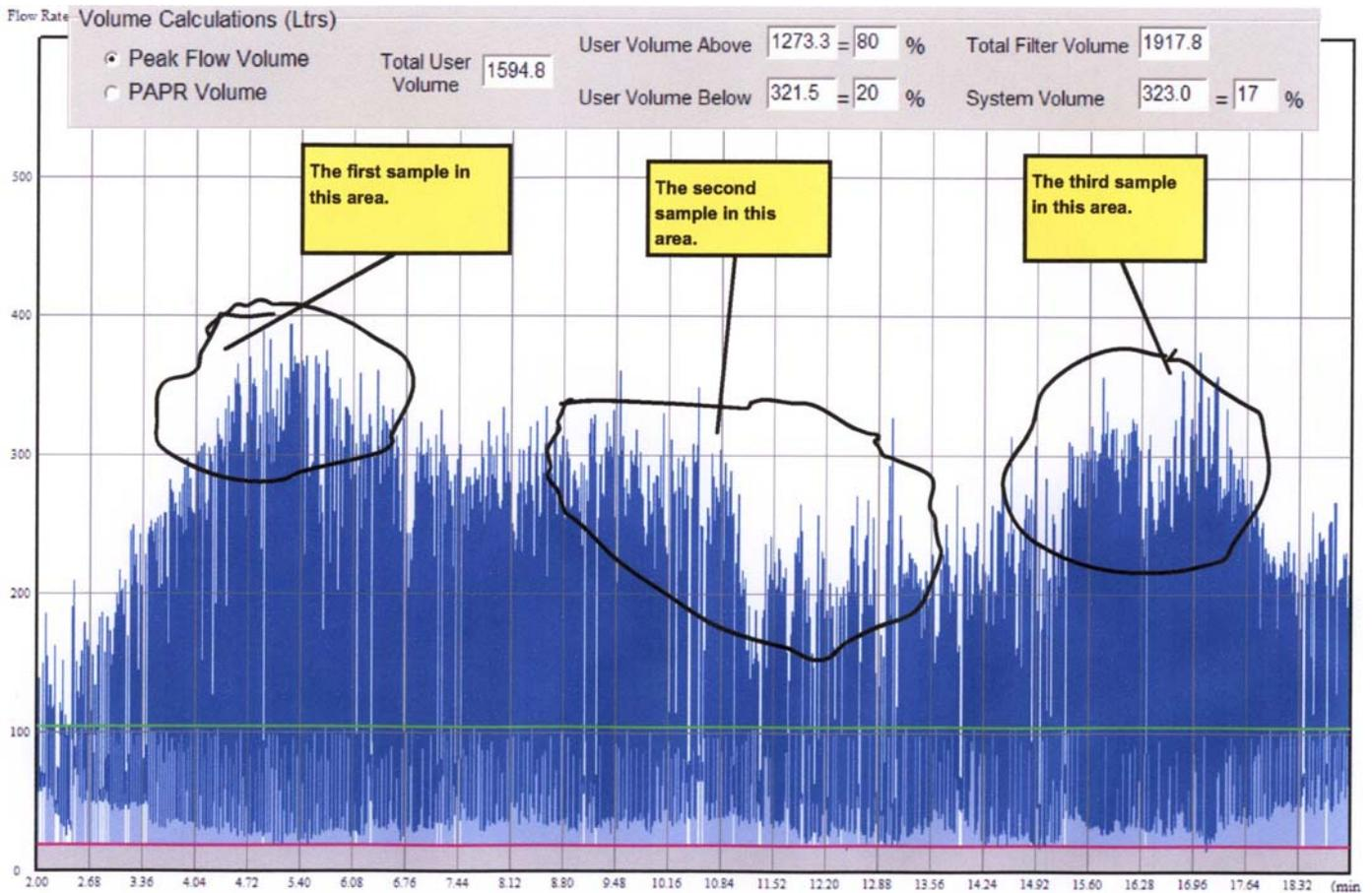
This person had a total system volume of 1,917.8 liter volume in the 16 minutes this graph represents. The total user volume is 1,594.8 liter minute volume (99.66 liters per minute). Of this total user volume, 1,273.3 liters or 80% flow faster than 85 lit/min (the rate used by NIOSH in testing filters for particle penetration and pressure drop).
