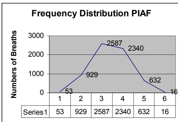
This shows a typical distribution curve. 75% of the peak flows are between 200-400 lit/min.
