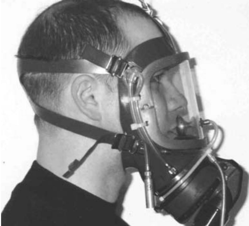
FIGURE 8: Open and size selecting ambient sampling devices fitted on SE400 facepiece. In-Mask probe and connection through facepiece visor is also shown. Note: inner-cup removed for purpose of photograph only.
