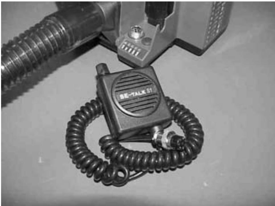
FIGURE 7b: SE400AT communication device connector
