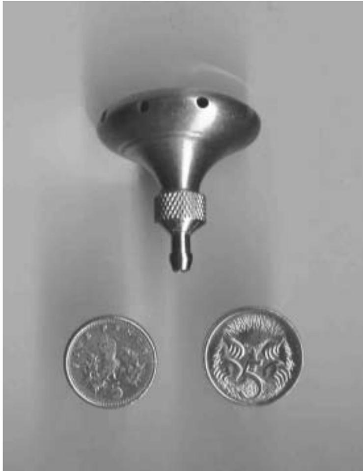
FIGURE 4: In-mask sampling probe. Shown with UK 5p and Australian 5 cent coins
