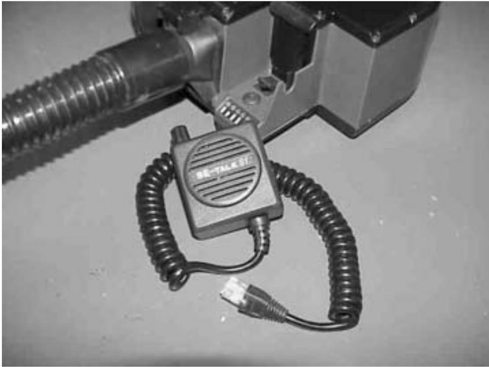
FIGURE 7a: SE400 communication device connector
