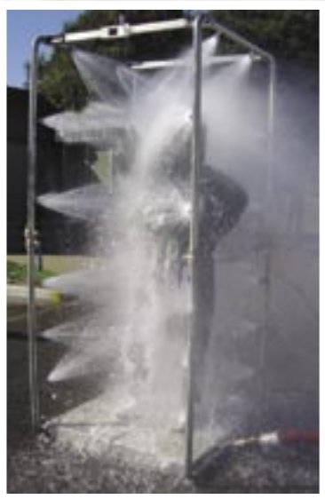
SE-shield can withstand wet decontamination without the need to remove the respirator even at very high water pressure
