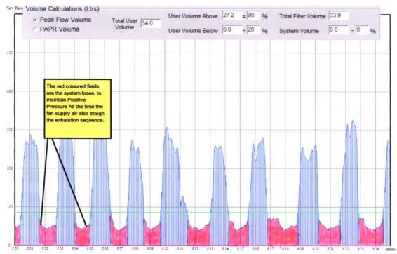
The function of an SE400AT is dependent not only on the flow requirement of the user but also on the pressure in the ori-nasal mask. The SE400AT adjusts its fan speed depending on the pressure in the ori-nasal mask to maintain Positive Pressure in the mask enclosure. Figure 3 shows a typical 15 second period of a subject. The
