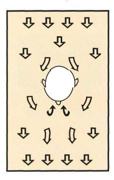
The same thing happens with air. If your ventilation system creates an even stream of air, a worker standing in that stream might act as the rock in the river. The air might swirl around the worker's face, actually drawing fumes from the contamination source back up towards the breathing region.
