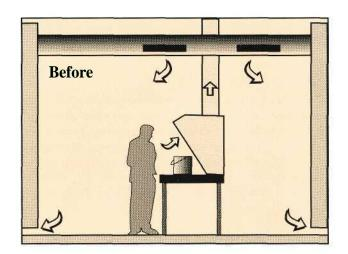
Before the installation of a work box, paint mixing was done at a work bench equipped with an exhaust hood running along the back end of the bench. Air input was through slots in an overhead duct. The exhaust air volume was around 1,000 m3/h. Additional air exhausts were located at floor and ceiling level. Measurements at the operator's face region detected xylenc, toluene and butanol in relatively low concentrations. Yet, the workers in the mixing room complained of frequent headaches.
