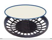
Snap the prefilter holder onto the front of the main filter.
