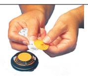
Pull out the inhalation membrane from inside the mask. Clean the membrane and the valve seat. Replace.
