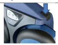
The fan will start and perform a self-test. During the test, the display symbols will light up, the beeper will sound, and the vibrator will buzz.
