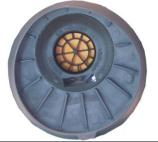
Remove the protective caps from the exhaust valves. Pull out the membranes and wipe clean. Wipe the valve seats before refitting the valves and replacing the protective caps.
