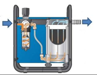
**IMPORTANT:** an air tool (spray gun, pneumatic nail gun etc.) counts as one user. The SR99 can deliver air to a maximum of three users OR air tools. If serving the maximum number of users or tools, the source of air (compressor/cylinder) must deliver at least 900 litres of air per minute.
