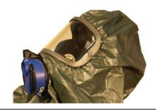
7. Attach the breathing hose to the face piece. If an exhalation valve shield (EVS, not shown) is to be used, fit this before attaching the hose.
