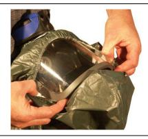
The hood should now be securely sealed around both the demand valve and the visor.
