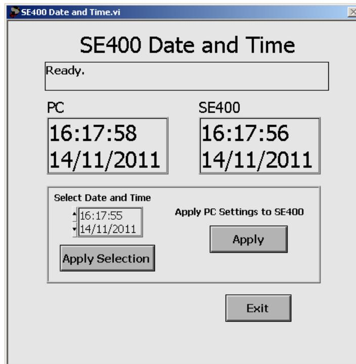
2. To set the SE400 date and time manually, at “Select Date and Time” enter the desired date and time and select <Apply Selection>. Wait for the updated SE400 date and time to be displayed. Select <Exit> to return to the previous screen.
