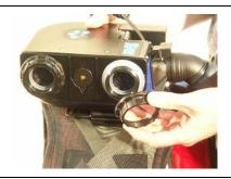
3. Insert the filter ports through the corresponding holes in the back of the suit. Refit the nuts and tighten firmly.
