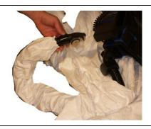
Connect the breathing hose to the mask, keeping the hose sleeve well away from the connection.
