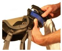
7. Pull the hose cover all the way up to the regulator connection.
