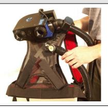
Undo the threaded nuts on the fan unit filter panel.
