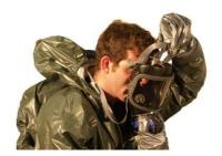
45. To increase comfort and minimise visor fogging, turn on the fan unit by pressing either the control button on the speaker unit or the power switch on the fan unit.
