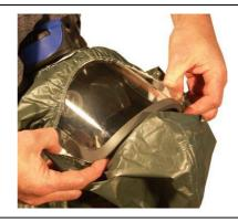
12. The hood should now be securely sealed around both the demand valve and the visor.
