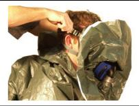
24. To increase comfort and minimise visor fogging, turn on the fan unit by pressing either the control button on the speaker unit or the power switch on the fan unit.
