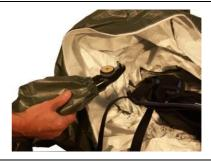
Tape the hose sleeve to the end of the hose, keeping the tape and sleeve well away from the membrane and the attachment surfaces of the hose connection.
