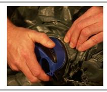
When finished, the elastic should sit snugly in the groove at the base of the valve.
