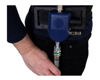
**10.1** Disconnect the compressed air hose from the control valve.
