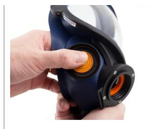
14.3 Press the new membranes onto the dowels.Carefully check that the membranes are in contact with the valve seats all round.
