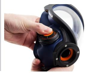
**14.4** Press the valve covers into place. A clicking sound indicates that the cover has snapped into place. Carry out leakage testing.
