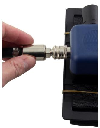
**6.1** Connect the breathing hose to the control valve outlet.
