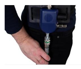
**9.2** Disconnect the compressed air hose from the control valve.
