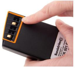
**3.1** Check that the gasket around the opening to the battery terminals on the underside of the battery is undamaged.
