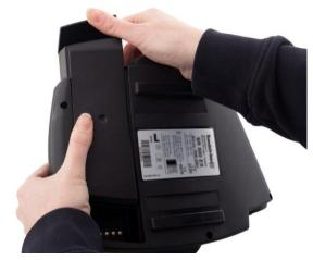
**1.2** Raise the battery cover a few centimeters and push with the thumb and withdraw the battery.
