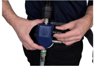
2.7 Use the control valve knob to set the air flow rate to suit your current work intensity. In the fully closed position (turn the knob anticlockwise), the flow is about 175 l/min, and in the fully open position (turn the knob clockwise), it is about 260 l/min.
