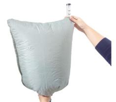
1.6 Place the head-top in the flow meter. Grip the bag to seal around the breathing hose. Grip the flow meter tube with the other hand, the tube will point upwards from the bag
