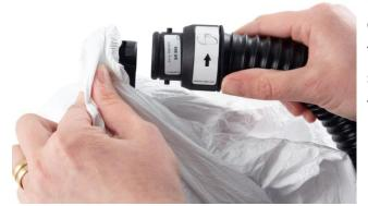
**6.3** Fit the new hose into the head harness in the reverse order. One hose connection is fitted with an O-ring. This end should be connected to the fan/compressed air unit.
