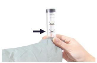
**2.2** Read the position of the ball in the tube. It should float level with or just above the marking on the tube.
