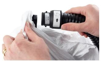
**6.2** Twist the hose and pull it out of the adapter.
