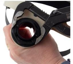
**7.3** Turn the locknut a quarter of a turn to remove it. Use polygrip pliers if the locknut is stiff to turn.
