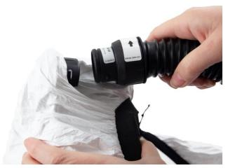
**7.2** Twist the hose and pull it out of the adapter
