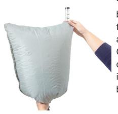
1.1 Place the facepiece in the bag and grip the opening of the bag so that it seals around the breathing hose. Grip the flow meter with the other hand and hold it so that it points vertically up from the bag.
