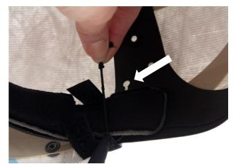
**5.9** Take the face seal rubber band and insert the knot into the keyhole opening in the head harness.
