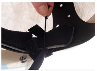
**5.2** Release the face seal rubber bands secured to the forehead band next to the Velcro tapes.
