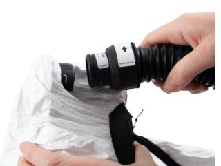
**6.2** Twist the hose and pull it out of the adapter.
