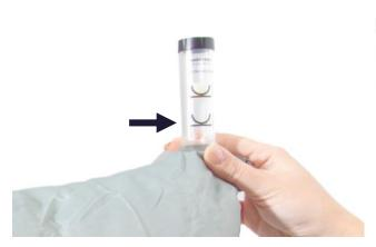
**1.2** Read the position of the ball in the tube. It should float level with or just above the marking on the tube.
