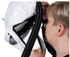
**3.1** Grip the hose mounting with one hand and the neck section of the hood with the other
