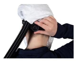
3.4 If necessary adjust the hood by means of the knob right at the back of the head harness. The knob is on the inside of the hood behind the hose. You can reach it without taking off the hood. Turn clockwise to tighten and counter clockwise to widen.
