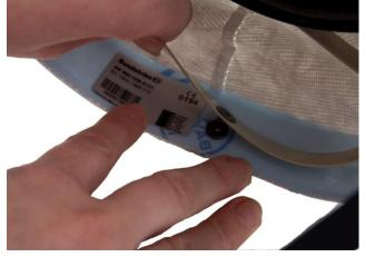
**5.7** Secure the hood by means of the press-studs at the top edge of the visor.
