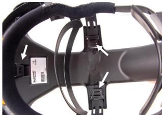
Assemble the new air-duct in reverse order or see the instructions in section 1. Assemble.
