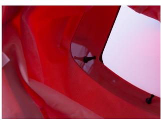
facing downwards, over the rubber studs. Bear in mind that the holes for the head harness screws must be oriented in the same direction as the hood and frame. Secure with the studs, possibly using a pair of pliers.
