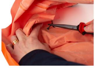
5.7 Bend the frame to the required shape. Align the vacant holes for the studs in the frame, hood and visor. Insert the studs and secure them by pulling the studs from the inside of the hood. The simplest procedure is to fit one stud at a time.
