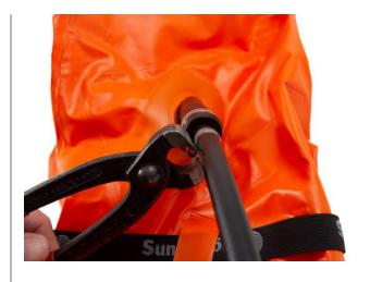
**6.3** Thread the hose clip supplied onto the new hose and connect the hose to the hose nipple of the hood. Secure the hose clip by means of the pincers.
