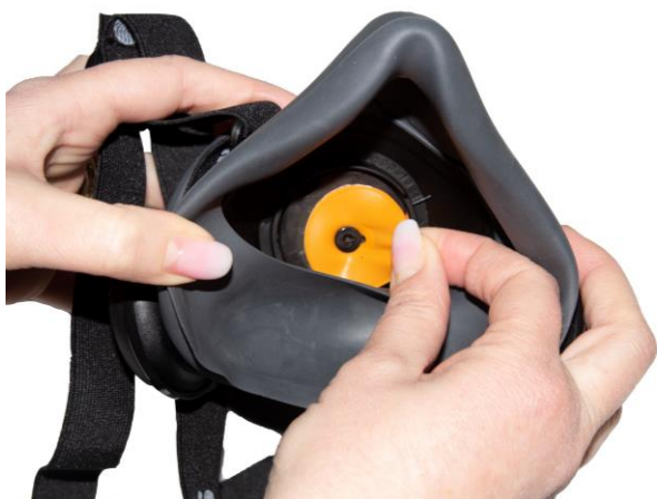
6.2 Fasten the new membrane on the pin.
