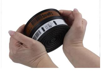
2.1 When using both gas filter and particle filter, the particle filter shall always be snapped onto the gas filter and the gas filter shall always be inserted in the filter holder. Press the filters together with your fingers placed around the outer edges of the filters until you hear a click.
