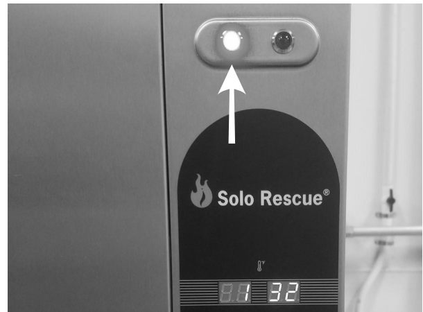
Figure 14: Once the program is complete, the green light is lit.
