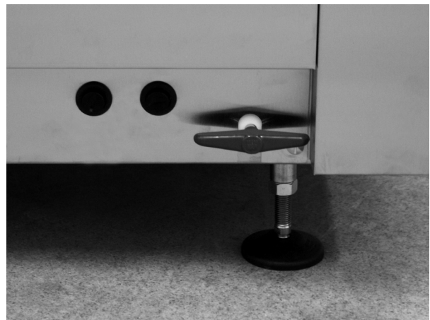
Figure 16: Access to the overheat protectors
