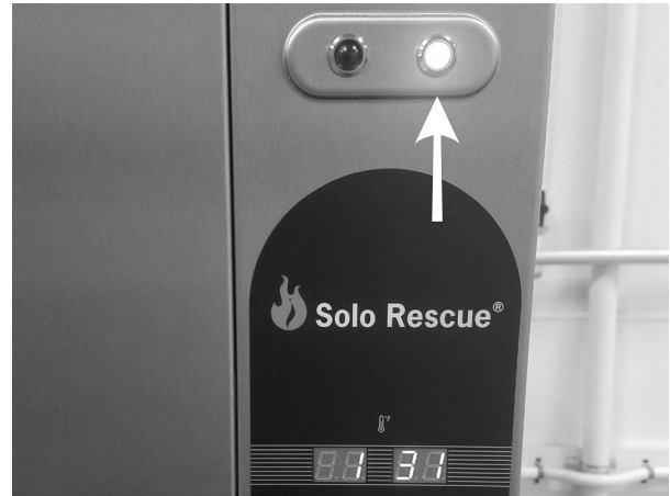
Figure 13: During the wash cycle the red indicator light will be on. Do not open the door when the red light is on.
