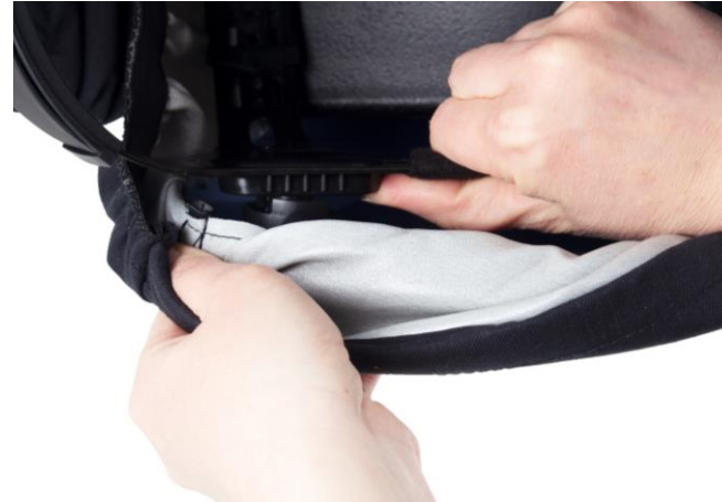
1.1 Height adjustment. How high the welding shield sits on the head.
