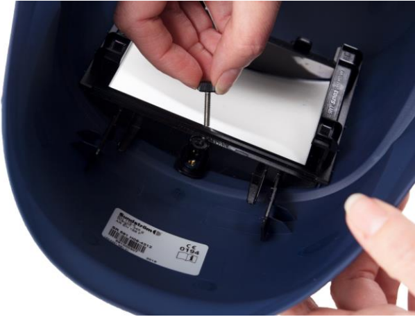
4.1 Loosen the screw in the holder for the welding filter.
