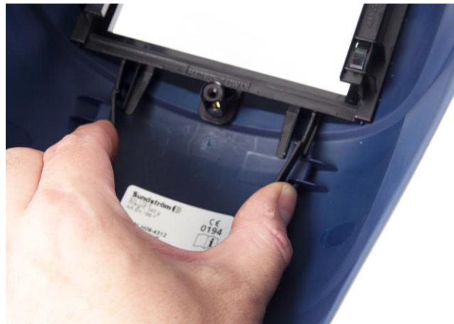
4.2 Release the holder for the welding filter.
