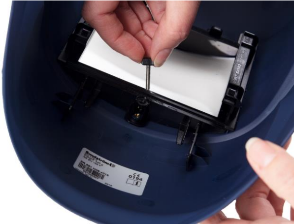
3.1 Loosen the screw in the holder for the welding filter.
